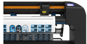
ORANGE Status = Hebe Andruckrollen an
